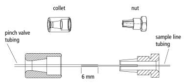
**b** Slide the pinch valve tubing over one end of the sample line tubing until approximately 6 mm of the sample line is inside the pinch valve tubing.
