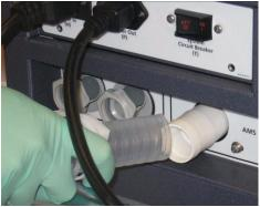
**NOTE** For optimal evacuation of aerosols, ensure that the tubing is securely connected at both ends.
