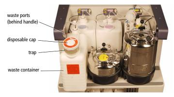
1 Disconnect the waste container's sensor and fluid line connectors from their respective ports on the fluidics cart.
