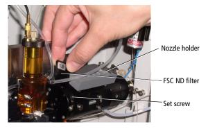
3 To reinstall the filter, slide it into the slot with the filter side down.
