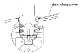
The amount and type of charge determines where the drop will be sorted. For example, in a four-way sort, drops with the most charge will be deflected into the outer streams, while drops with less charge will be deflected into the inner streams.
