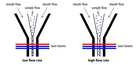
Ideally, you want the core stream at its minimum diameter so that cells pass through the laser beam in a single-file stream. However, depending on your application, a lower resolution might be acceptable in order to acquire the data more quickly. For example, a higher flow rate is generally used for qualitative measurements such as immunophenotyping—the data is less resolved but is acquired more quickly. A lower flow rate is generally used in applications where greater resolution is critical.
