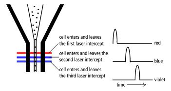
The delay factor in BD FACSDiva software is used to realign the signals so they can be measured and displayed on the same time scale. Note that signals are aligned with respect to the blue laser, so the red laser signals always have a negative delay value.
