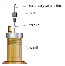
**3** Ensure that a cone-shaped ferrule is attached to the sample line.
