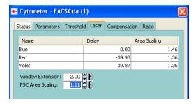
**b** Adjust the FSC area scaling factor until the FSC-A signal matches the FSC-H signal. See Figure 4-16.
