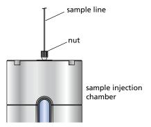
**4** Push the sample line down so the end is below the bottom of the sample injection chamber.
