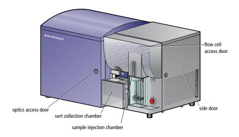
To view the fluidics components, open the side door and lift the flow cell access door. To view the optics components, open the optics access door. The power panel and connectors are found on the left side of the cytometer. Other electronic components are embedded within the cytometer and do not need user adjustment.
