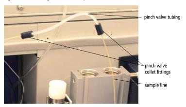
3 Unscrew the nut on the black collet fitting at each end of the tubing, and pull the pinch valve tubing out of both fittings.
