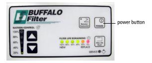
**6** Press the up or down arrow button to set the suction control rate to 20%.
