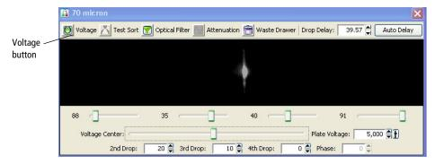
Make sure the center stream image does not move after the plates are turned on. Major movement of the center stream could indicate that the plates or area around the plates needs cleaning.
