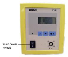
2 Use the up or down arrow keys to set the required temperature.
