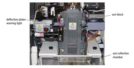
Additional aerosol removal is provided by the BD<sup>TM</sup> Aerosol Management Option (AMO). The AMO is an optional device that evacuates the sort collection chamber during sorting. The AMO is equipped with a 0.01-um pore ultra-low penetrating air (ULPA) filter to trap aerosolized particles.
