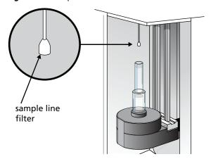
5 Install the sample line filter by sliding it onto the end of the line, then click Done. See Figure 6-23.
