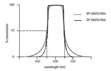
In the detector arrays, DF filters block high-intensity laser light and filter the remaining light to ensure that only the required wavelengths reach their intended detector. For example, in the octagon array, PMT-A has a 780/60 DF filter in front of it, which transmits light of 750–810 nm. Thus, the only wavelengths that will reach the A detector are those between 750 and 810 nm.
