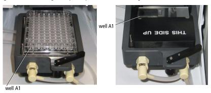
Sorting starts on the front left corner of the device (A1 location), and proceeds from front to back, and then from left to right, sorting in a serpentine motion. Thus, for a plate, sorting proceeds from well A1–A12, B12–B1, C1–C12, and so on.
