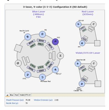
Figure B-4 Three-laser system configuration with Near UV laser
