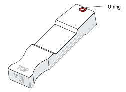
When installing or removing the nozzle, make sure the O-ring is in place before proceeding. Look at the O-ring in the nozzle with a magnifier or under a microscope to confirm it is positioned correctly.
