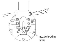
**3** Insert the new nozzle into the flow cell.
