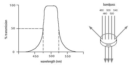
Figure 2-9 Light transmittance by bandpass filters
