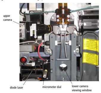
Special image-processing software allows you to view the stream images from each camera within separate windows in BD FACSDiva software. See Sorting on page 60 for more information about viewing the streams and to learn how Accudrop components are used to determine the drop delay.
