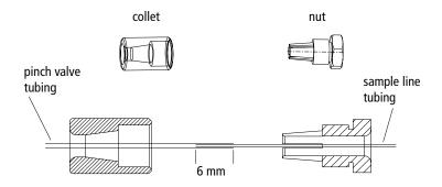
5 Install the new pinch valve tubing into the slot in the pinch valve.
