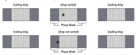
Decreasing the Phase Mask to 8 allows more drops to be sorted. However, because the target particle is closer to the edge of the drop, there is more variability in drop trajectory (Figure 2-23).
