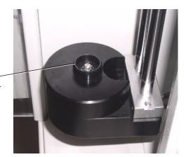
Apply lubricant to outside beveled edge of tube holder base.
