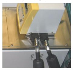
5 Connect the insulated hoses from the recirculating water bath to the cytometer control panel.
