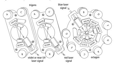
At installation, the octagon and trigon arrays are set up with the filter and mirror combinations shown in Table 8-7 on page 258. You can rearrange these configurations according to the type of fluorochromes in your experiment.
