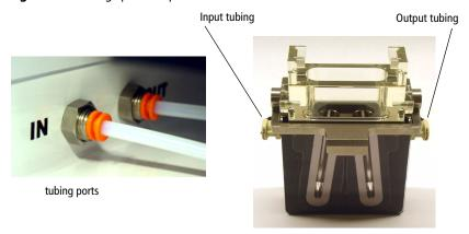
If you need to remove the tubing, push in the orange collar as you pull the tubing out of the port.
