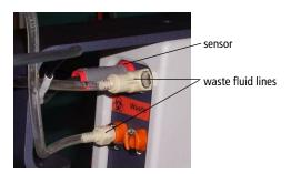
The waste container can become pressurized when the cytometer is running. Always disconnect the container from the fluidics cart before you empty it. Wait at least 1 minute for pressure to dissipate before you open the container.
