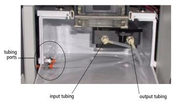
If you need to remove the tubing, push in the orange collar as you pull the tubing out of the port.
