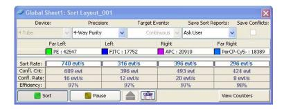
**NOTE** When the Sweet Spot is on, sorting pauses automatically if the Drop 1 or Gap values are out of range. This ensures that sorting occurs only under the proper breakoff conditions. If a more severe problem such as a clog is detected, the stream shuts off and sorting stops. The deflection plates shut off, the aspirator drawer closes, and the sample tube is unloaded. To clear a clogged nozzle, see Cleaning the Nozzle on page 216.
