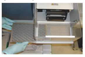
2 Install a new air filter in the door.
