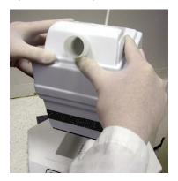
Push down on the filter to ensure that it is seated against the bottom of the filter chamber (Figure C-9 on page 293).
