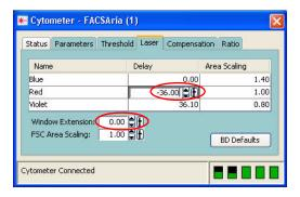
**d** Adjust the laser delay value until the maximum APC-A signal is achieved.
