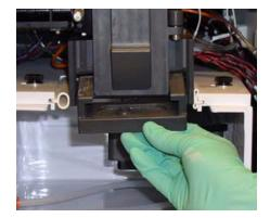
**2** Ensure that an air filter is installed in the sort collection chamber door.
