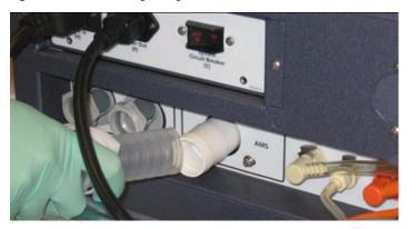
**3** Remove the spring-loaded filter hold-down.
