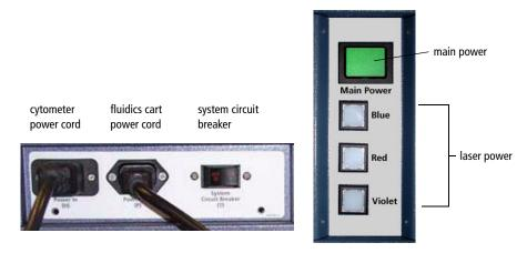
The cytometer circuit breaker is located next to the fluidics cart power cord (Figure 1-21). The switch will need to be reset if there is a power surge in the laboratory.
