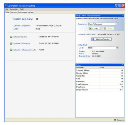
Werify that the bead lot information under Setup Beads matches the Cytometer Setup and Tracking bead lot.
