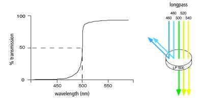
Dichroic filters that are used to direct different color light signals to different detectors are called dichroic mirrors or beam splitters.
