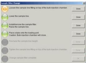
3 Loosen the sample line fitting nut at the top of the injection chamber to allow the sample line to slide freely through the fitting. See Figure 6-22 on page 221.
