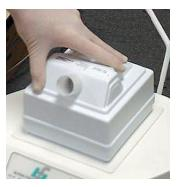
**NOTE** For optimal evacuation of aerosols, the filter must be completely seated in the evacuator filter well.
