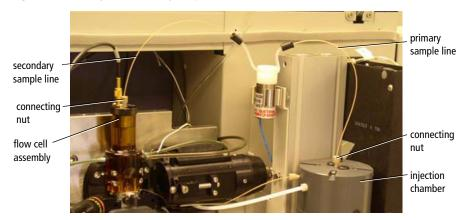
To withstand the high pressures generated by the BD FACSAria II flow cytometer, the sample lines are attached using a two-piece compression fitting, where a cone-shaped ferrule is compressed onto the tubing as the connecting nut is tightened.
