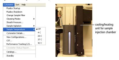
The cooling/heating unit is designed to maintain the temperature of a sample tube. It is not designed to cool or heat the sample. It takes approximately 45 minutes to reach the required temperature inside the chamber, during which time the chamber must be kept closed.
