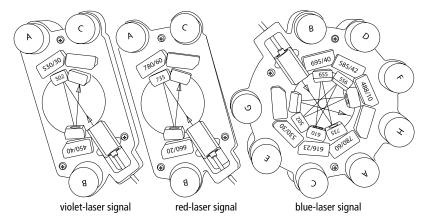
Each detector array houses dichroic and bandpass filters, which steer and filter the emitted light, and photomultiplier tubes (PMTs), which detect light signals.
